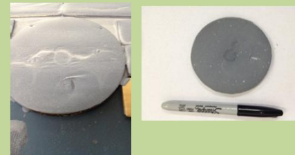
Cast coated (left) and sintered (right) YSZ on bond coat/substrate
